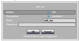
8 Press ▲ or ▼ to highlight the **Password** field, then press **ENTER**. An on-screen keyboard appears.
